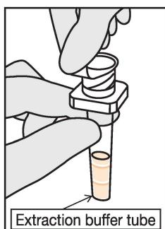
Remove the aluminum sealing cap from the extraction buffer tube, while taking care not to spill the liquid.
