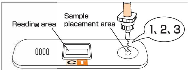
Hold the middle of the tube with the fingers and dispense **3 drops** of the sample.
