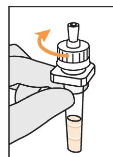
Firmly attach the nozzle (with a filter) provided in the kit to the top of the extraction buffer tube.
