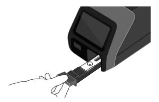
4. Sofia 2 will start automatically and display the progress as shown in the example below. In WALK AWAY Mode, the test results will be displayed on the screen at 15 minutes. In READ NOW Mode, the test results will be displayed on the screen within 1 minute. See Interpretation of Results section.
