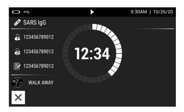
For example: This display shows that the test in WALK AWAY Mode has 12 minutes, 34 seconds remaining. Sofia 2 will read and display the results at 15 minutes.
