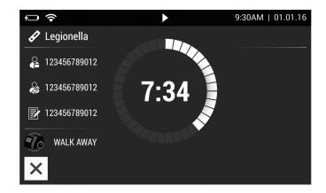
For example: This display shows that the test in WALK AWAY Mode has 7 minutes, 34 seconds remaining. Sofia 2 will read and display the results after 10 minutes.
