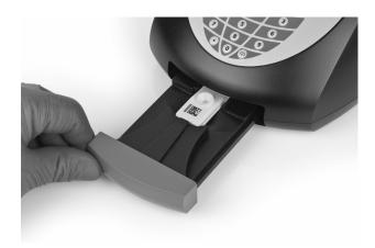
5. Sofia will start automatically and display the progress. In WALK AWAY Mode, the test results will be displayed on the screen within 10 minutes. In READ NOW Mode, the test results will be displayed on the screen within 1 minute. See Interpretation of Results section.
