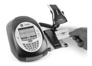
2. Input Patient ID or Order # using the barcode scanner or manually enter the data using the key pad.
