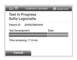
For example: This display shows that the test in WALK AWAY mode has 7 minutes, 13 seconds remaining. Sofia will read and display the results after 10 minutes.
