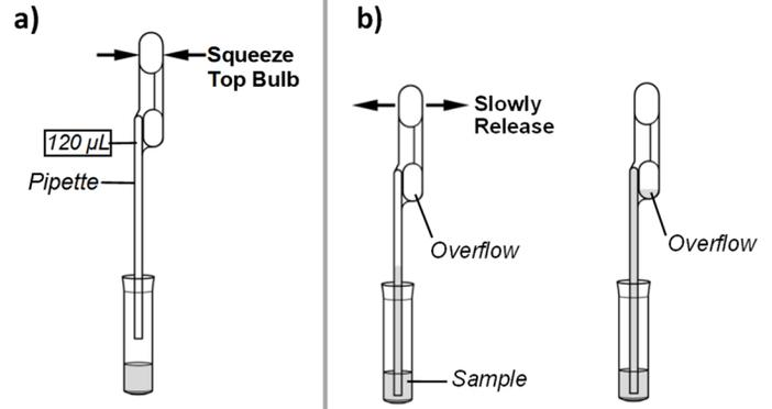
10. Empty the contents of the Pipette into the Test Cassette sample well by firmly squeezing the top bulb. Extra liquid left over in the overflow bulb should be left behind.
