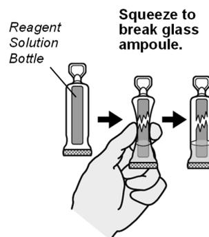
3. **Vigorously** shake the Reagent Solution Bottle **5 times** to mix the solutions. Solution should turn green after the ampoule is broken.
