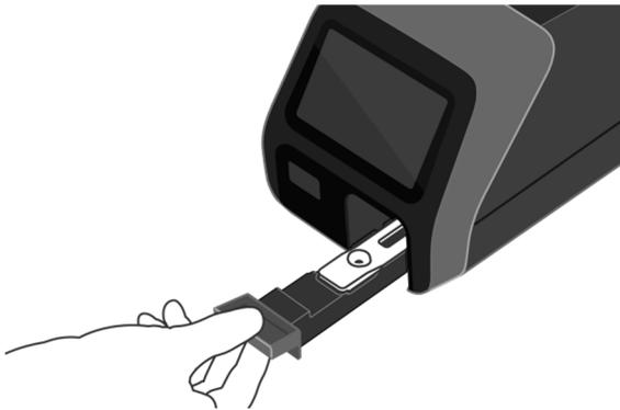
5. Sofia 2 will start automatically and display the progress, as shown in the example below. In WALK AWAY Mode, the test results will be displayed on the screen in approximately 5 minutes. In READ NOW Mode, the test results will be displayed on the screen within 1 minute. See Sofia 2 Interpretation of Results section.
