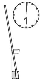
7. **Vigorously** mix the solution again by plunging the Swab **5 times** in an up and down motion in the Tube.
