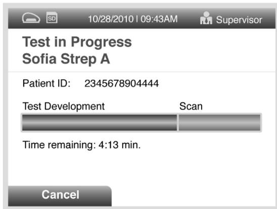
*For example: This display shows that the test in WALK AWAY Mode has 4 minutes, 13 seconds remaining. Sofia will read and display the results after 5 minutes.*
