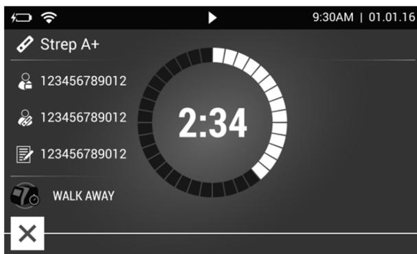
***For example: This display shows that the test in WALK AWAY Mode has 2 minutes, 34 seconds remaining. Sofia 2 will read and display the results after 5 minutes.***
