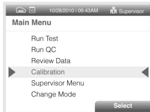
2. Following the prompts, insert the Calibration Cassette into Sofia and close the drawer. Sofia performs the Calibration Check automatically within two minutes with no user input required.
