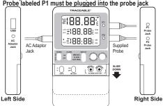
labeled "P1" and probe labeled P2 must be plugged into the probe jack labeled "P2".
